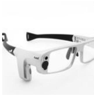
**Figura 2.2:** Mobile eye tracking - Tobii Glasses [13].
